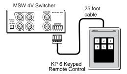
Figure 3 — KP 6 application (with 5-pole captive screw connector)
